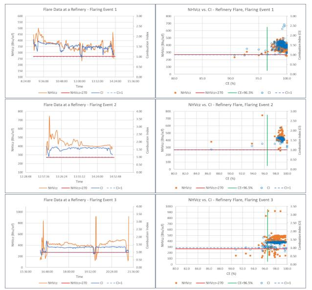
**Figure 7:** Comparison of the NHVcz method and the CI method based on a flare study at an anonymous refinery in the U.S.
