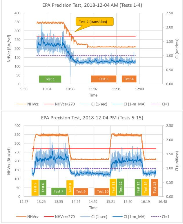
**Figure 3:** Continuous monitoring of the test flare at John Zink test facility using NHVcz and CI during Day 1 of the EPA precision test in 2018.
