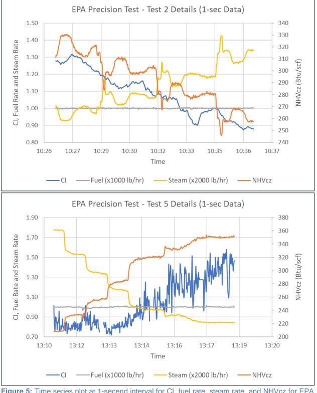
**Figure 5:** Time series plot at 1-secend interval for CI, fuel rate, steam rate, and NHVcz for EPA Precision Test 2 (transition from high CE to low CE and Test 5 (transition from low CE to high CE).
