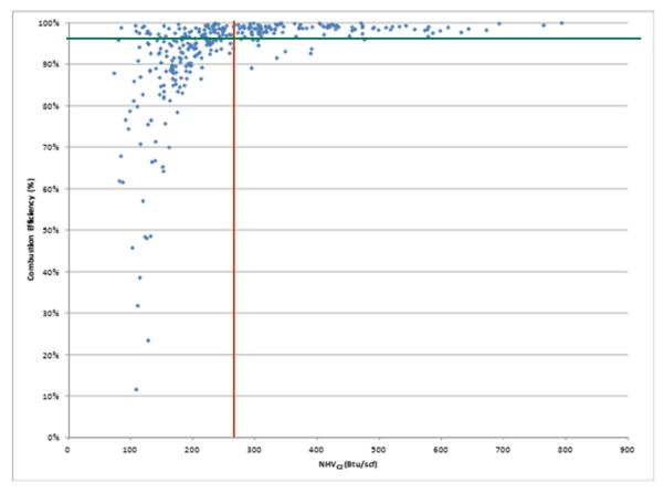
**Figure 1:** Relationship between flare CE and NHVcz as well as regulatory target for CE (>96.5%) and compliance threshold for NHVcz (>270 BTU/scf). Source: Ref. USEPA, 2012, p. 3-33. The red vertical line (NHVcz=270 BTU/scf) and green horizontal line (CE=96.5%) are added by author.
